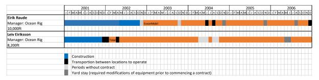
From the delivery of the rigs from the construction yard in the beginning and end 2002 respectively, the rigs have operated on multiple contracts (orange blocks). The blue blocks indicate construction, the black blocks indicate transportation between locations to operate, the light grey blocks indicate periods without contracts and the dark grey blocks indicate a yard stay (required modifications of the equipment prior to commencing on a contract).
